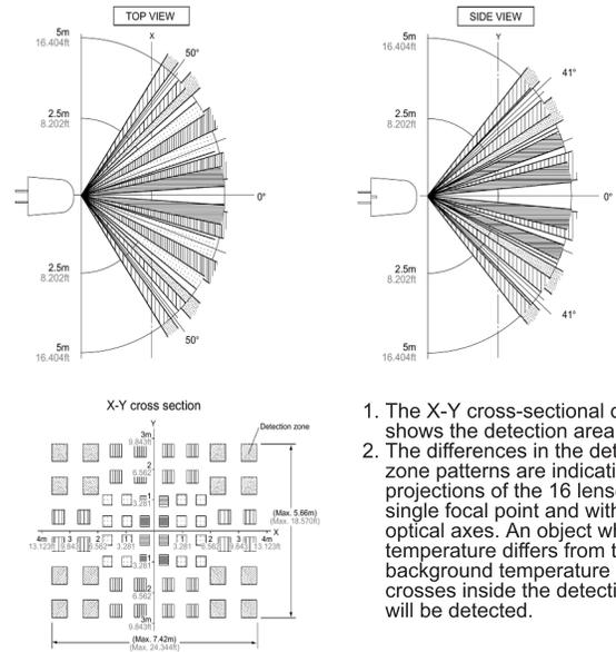
1. The X-Y cross-sectional diagram shows the detection area.
